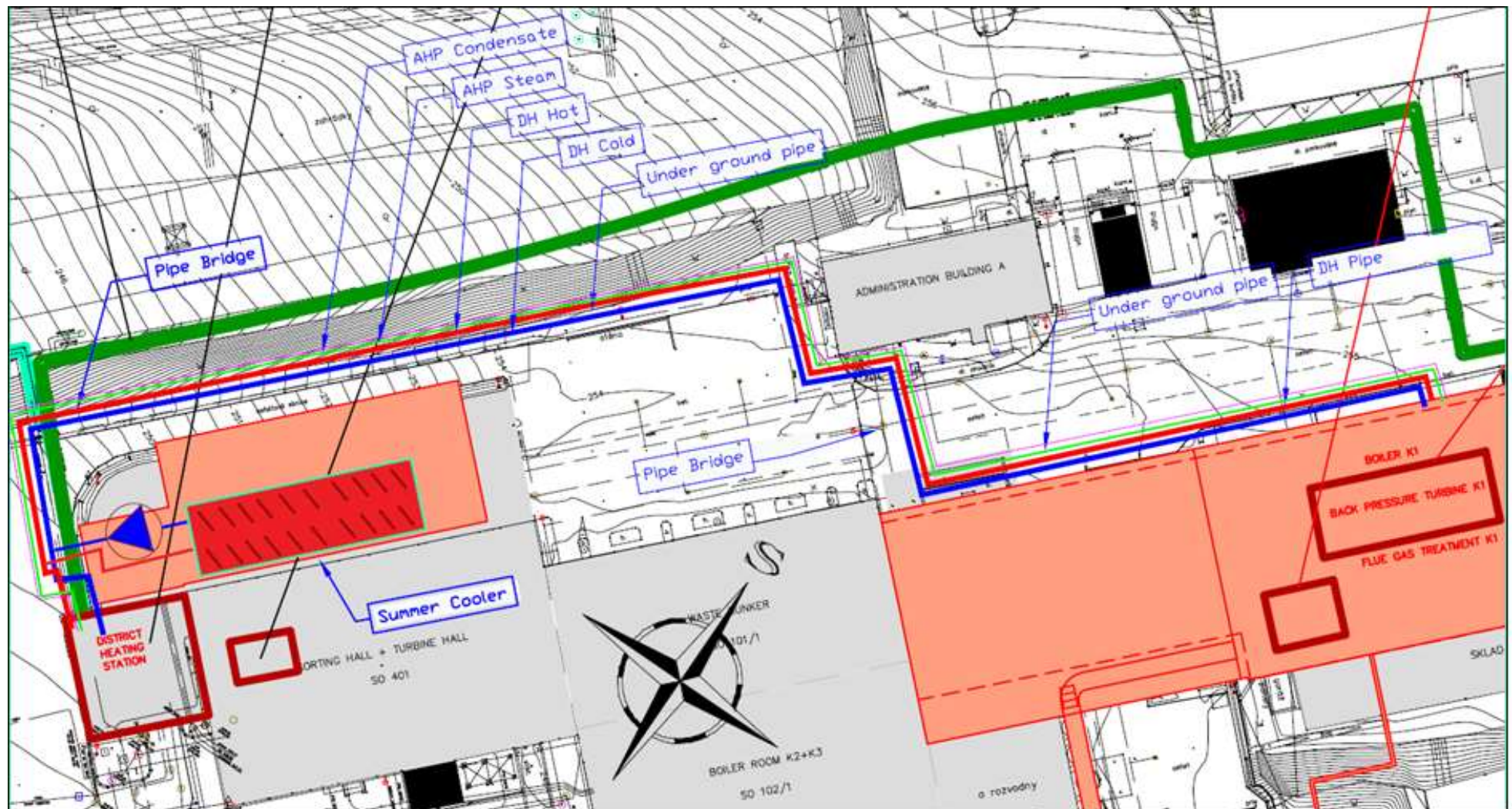
Figure 2, Suggested pipe routing between the Line (Line K1) and existing DH building. "S" is towards the north.
